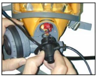
2. Insert the microphone portion into the port. The nickel microphone wires may need to be bent slightly to install. Tighten thumb screws (hand tight only).
