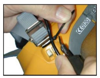
9. Loosely secure the cable to the buckle of the full face mask with the supplied tie wrap as shown. **CAUTION:** Be sure the tie wrap does not bind the cable so it can slide freely. Improper installation may cause the mask to leak.
