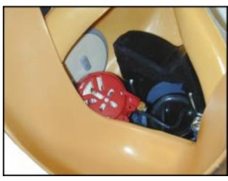
3. Once the microphone is inside the port, carefully position the microphone within <sup>1</sup>/<sub>4</sub>" from the diver's lips. This will place the microphone at the left corner of the diver's lips. The Hot Mic is shown above, other microphones are available.
