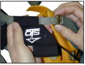
6. Insert the AGA straps through the top and bottom slots of the EHA-1. Re-assemble the AGA straps into the mask.
